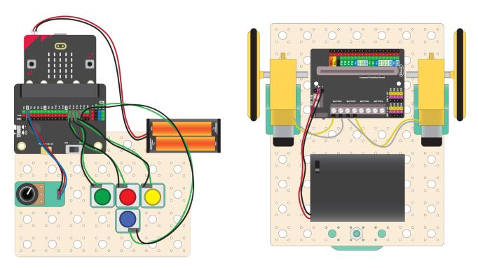
For the speed control you will add a **potentiometer** to the remote control. This is an **analogue input device**. By turning the knob, you can get different values from 0 to 100 which can be used to set the speed. When we read the value from the potentiometer on the controller, we need to send the value across to the robot, so it can adjust its speed:
